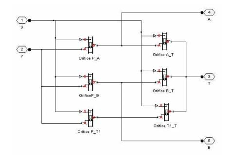
The Orifice with Variable Area Round Holes blocks have been used as a variable orifice in this model. Port T1 corresponds to an intermediate point between ports P and T.
