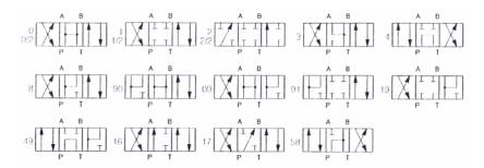
Most of these patterns can be implemented by selecting initial orifice openings in the four-orifice valve configuration shown in the previous section, in the
